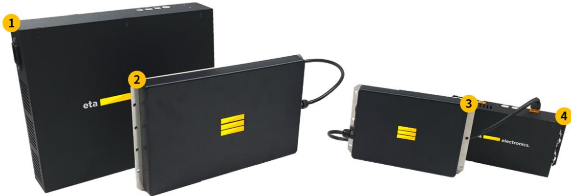
1 Tx control module 2 Tx coil module 3 Rx coil module 4 Rx control module
